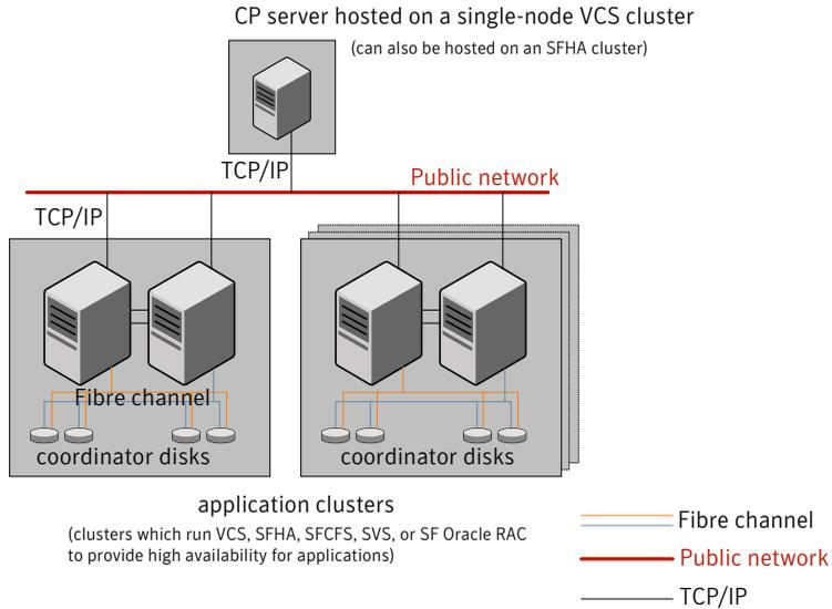
Figure 7-6 displays a configuration using a single CP server that is connected to multiple application clusters.
