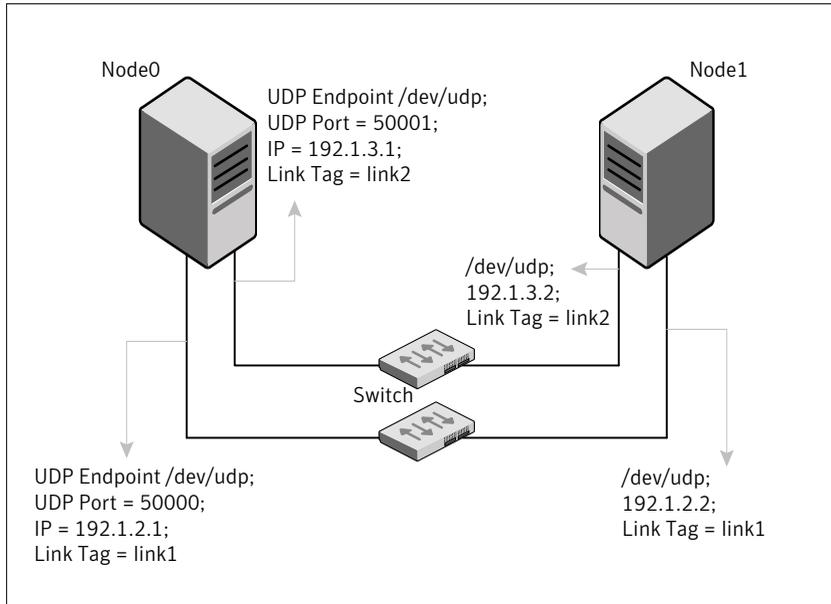
The configuration that the `/etc/llttab` file for Node 0 represents has directly attached crossover links. It might also have the links that are connected through a hub or switch. These links do not cross routers.
