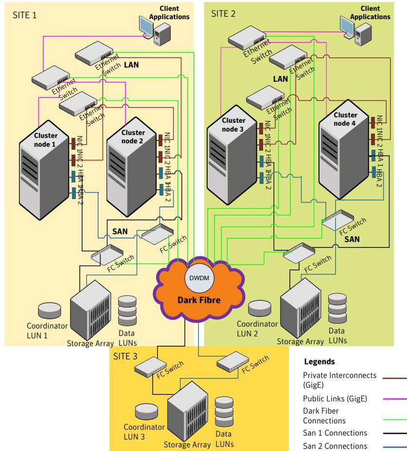
Although a Coordination Point (CP) server is not used in the current example, it can also be used instead of a third site for a coordinator disk.
