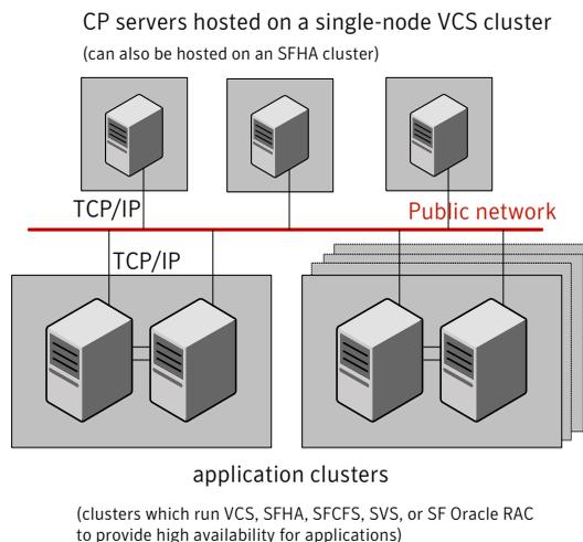
Figure 7-5 displays a configuration using a single CP server that is connected to multiple application clusters with each application cluster also using two coordinator disks.
