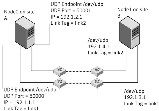
The configuration that the following `/etc/llttab` file represents for Node 1 has links crossing IP routers. Notice that IP addresses are shown for each link on each peer node. In this configuration broadcasts are disabled. Hence, the broadcast address does not need to be set in the `link` command of the `/etc/llttab` file.
