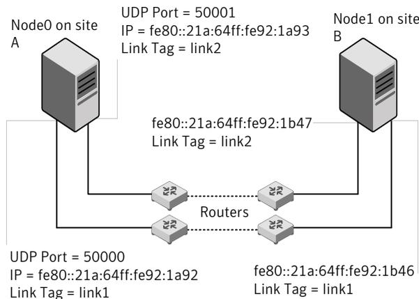
The configuration that the following `/etc/llttab` file represents for Node 1 has links crossing IP routers. Notice that IPv6 addresses are shown for each link on each peer node. In this configuration multicasts are disabled.
