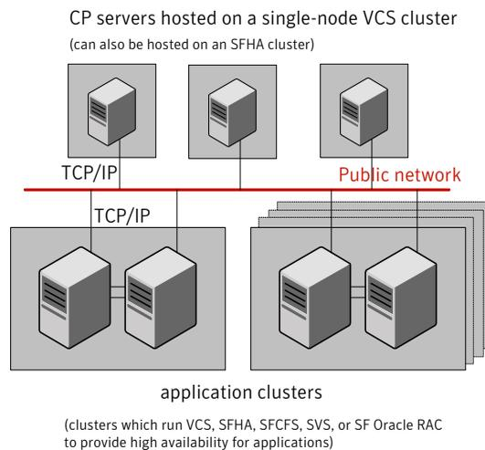
Figure 3-6 displays a configuration using a single CP server that is connected to multiple application clusters with each application cluster also using two coordinator disks.
