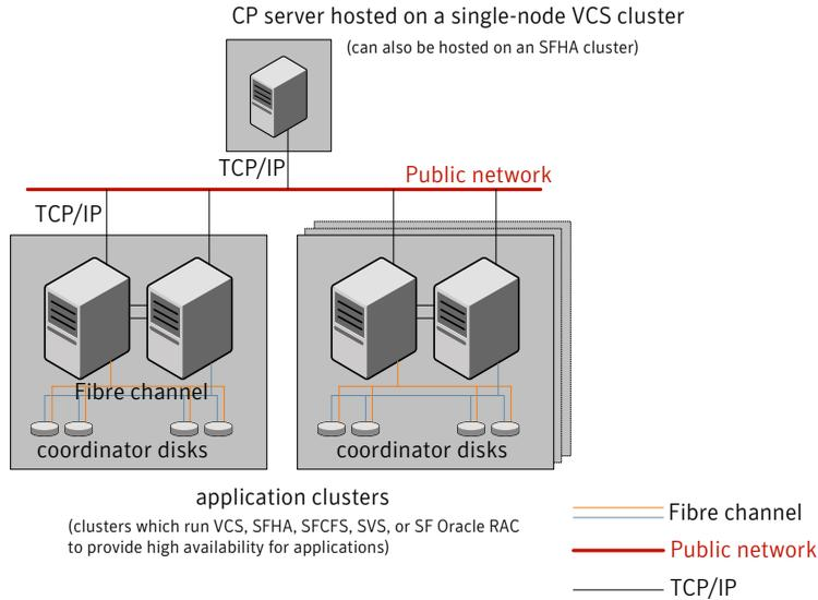
Figure 3-7 displays a configuration using a single CP server that is connected to multiple application clusters.
