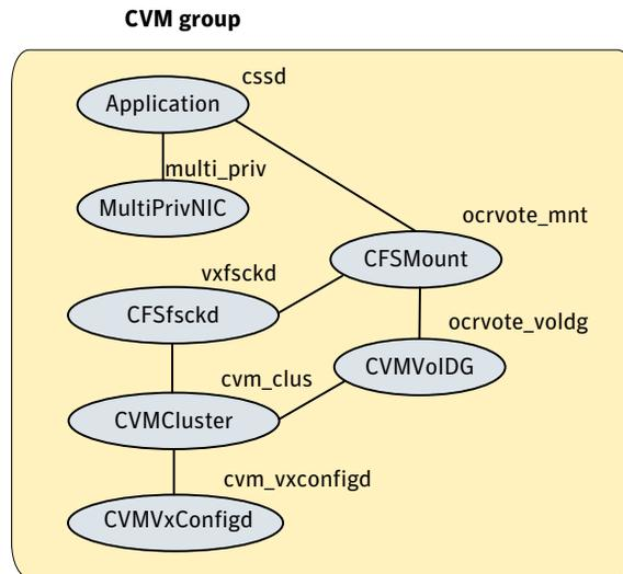
Figure 20-5 illustrates a sample service group configuration in the absence of the VCS Oracle agent for multiple database configurations.
