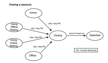
When the resource is disabled (Enabled=0), the agent stops Periodic Monitoring and the *close* entry point is invoked. When the *close* entry point succeeds or times out, the resource is placed in the Detached state.
