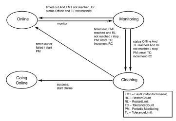
This diagram describes the activity that occurs when a resource faults and the RestartLimit is not reached. When the *monitor* entry point times out successively and FaultOnMonitorTimeout is reached, or monitor returns offline and the ToleranceLimit is reached, the agent invokes the *clean* entry point.
