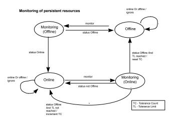
For a persistent resource in the Online state, if *monitor* returns a status of offline and the ToleranceLimit is not reached, the resource stays in an Online state. If *monitor* returns offline and the ToleranceLimit is reached, the resource is placed in an Offline state and noted as FAULTED. If *monitor* returns "not offline," the resource stays in an Online state.
